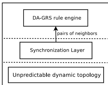
Fig. 3. Abstraction of the synchronization layer
